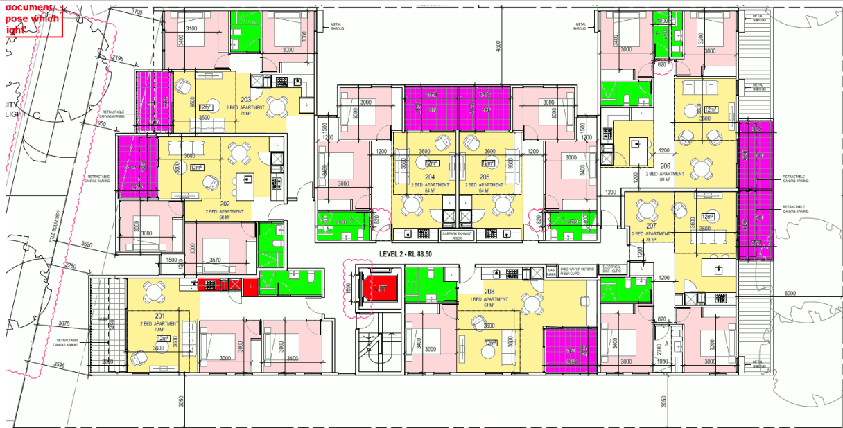
L2 Bed rooms, living areas, Corridor kitchen, bathrooms, undersize balconies
